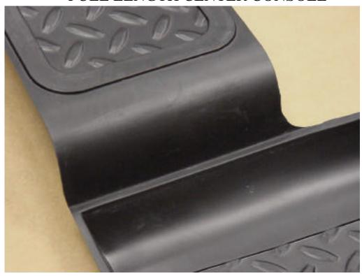
TRIM ALONG INTERSECTION OF THE "STEP" IN THE PART AND THE PORTION OF THE LINER THAT CONTINUES OVER THE HUMP. THIS WILL LEAVE A "LIP" ON THE TRIMMED LINER AS SHOWN IN THE PHOTO BELOW.
